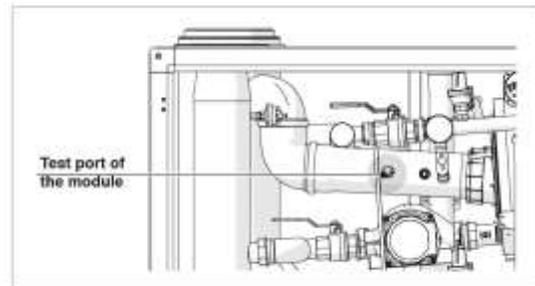
Fig.19 Test Port for Combustion Analysis (available on each individual heat exchanger)
